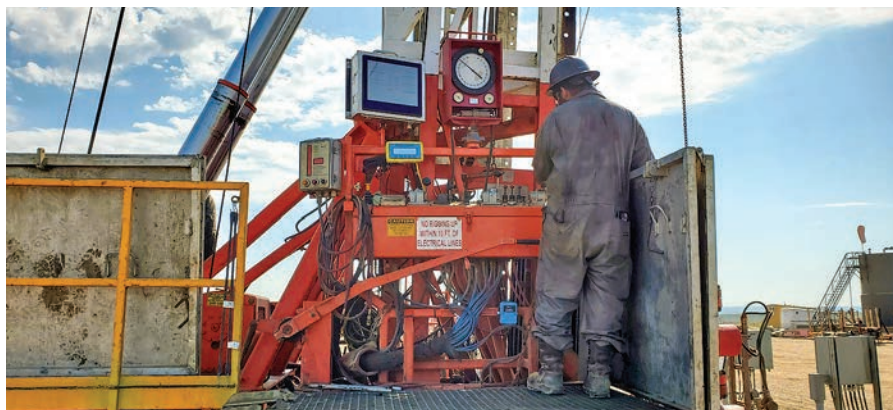
Fig. 1. The rig data display and field monitor ensure that all relevant information is available to the rig operator and remote users.
